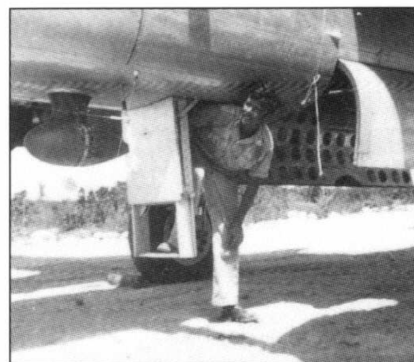
Lt Voelker of the 445th BS climbs out of the forward entry/exit hatch, with open bomb-bay doors behind him (Richard Krause)
