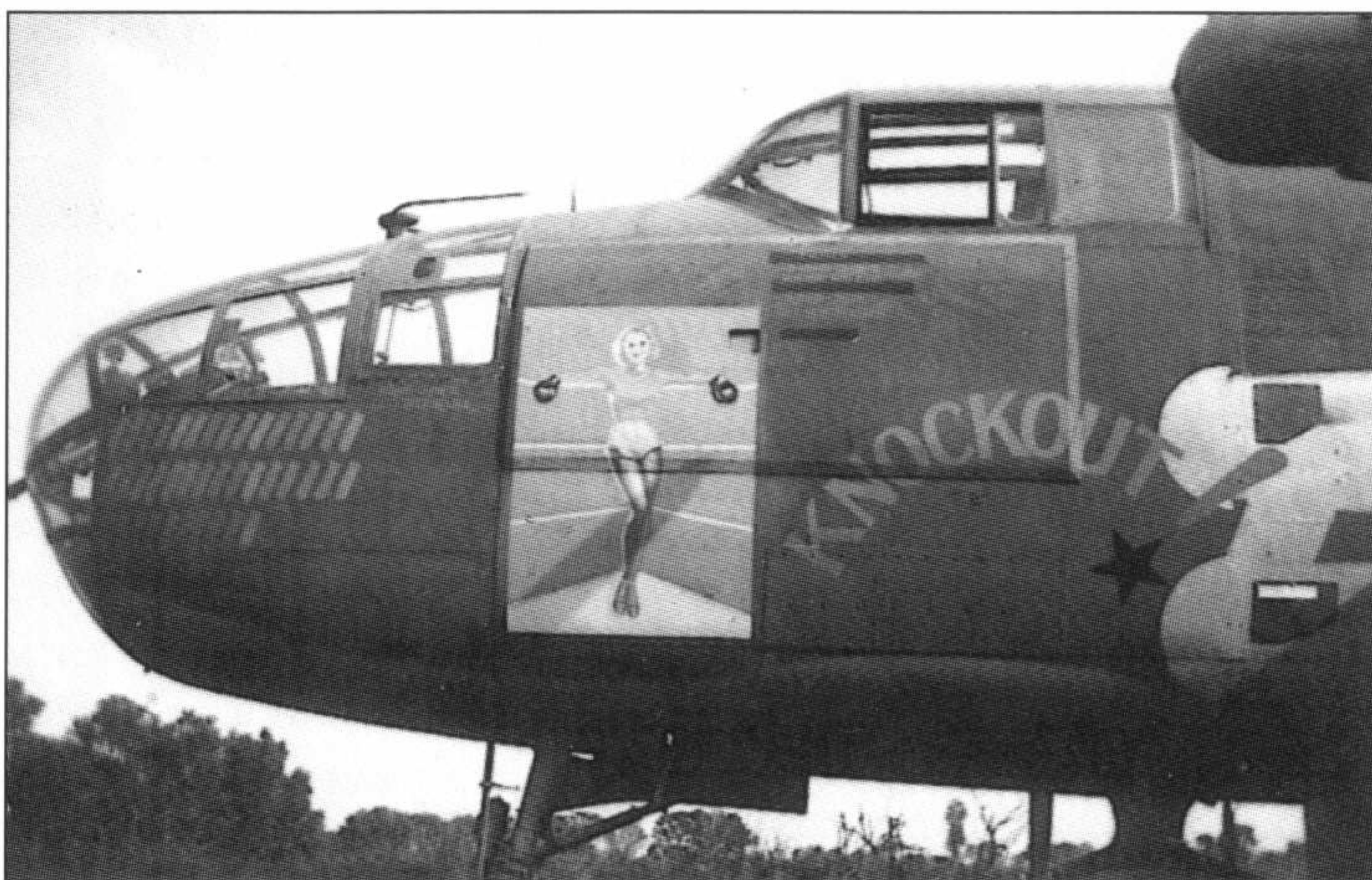
Another 340th BG machine, B-25J-1 43-4080/9S' KNOCKOUT! was assigned to the 489th BS. Note that its blister gun packs have been removed from the fuselage sides, revealing bare aluminium skinning. The 340th did little strafing in the MTO, resulting in the weighty gun packs being deemed surplus to requirements ( Harry D George Jr )
