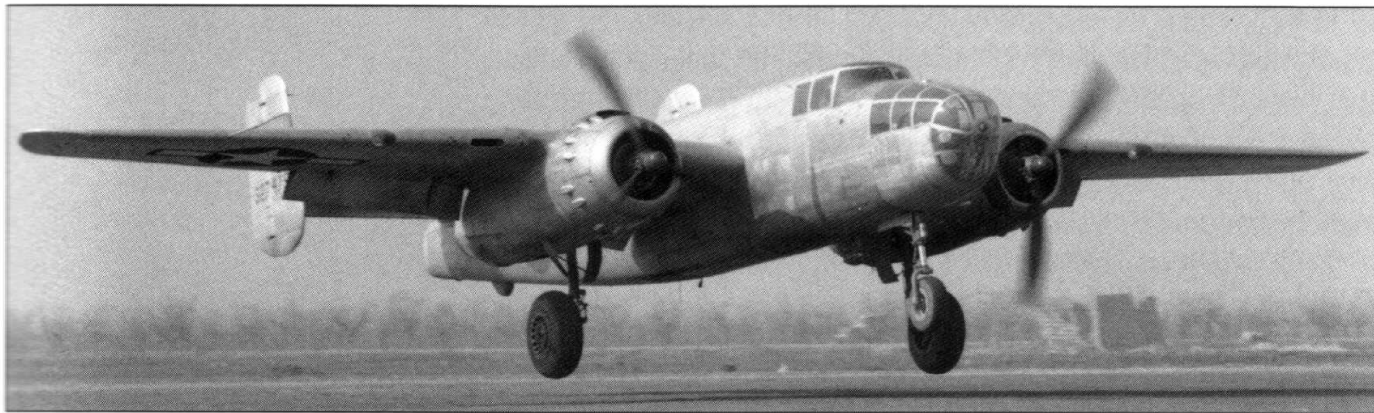
B-25J-1 43-27475 is just moments away from returning to the 310th BG's Fano base on the Adriatic coast in late 1944. Note that this machine lacks both its upper turret and its nose-mounted 0.50 cal machine gun (Norm Taylor Collection)
